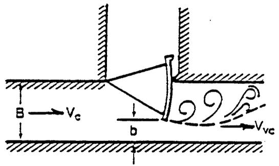
Figure 8.26. Culvert control valve ("reverse" tainter gate).
