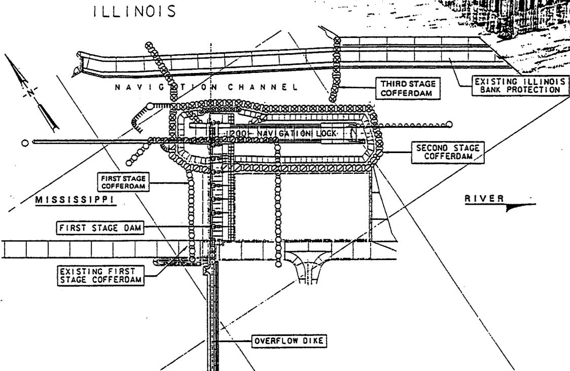
Figure 8.6. Three-stage cofferdam scheme, Replacement for Lock and Dam 26, Mississippi River.
