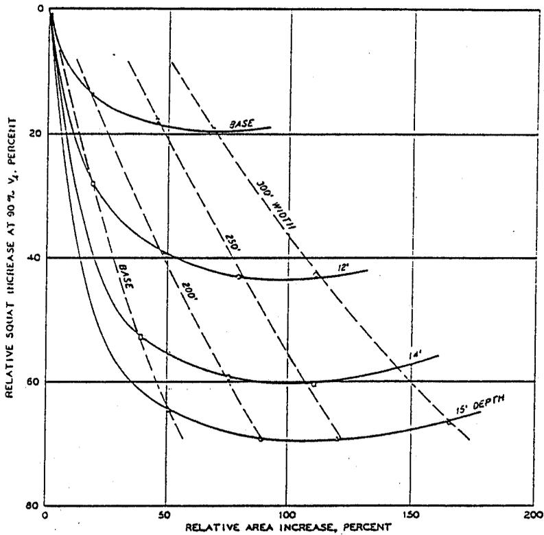
Figure 9.23 Effect of canal size on tow squat at 0.9 V, (Huvel, 1980).
