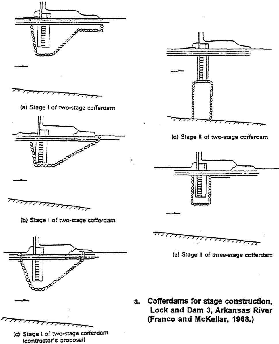
Figure 8.5. Cofferdams for stage construction.
