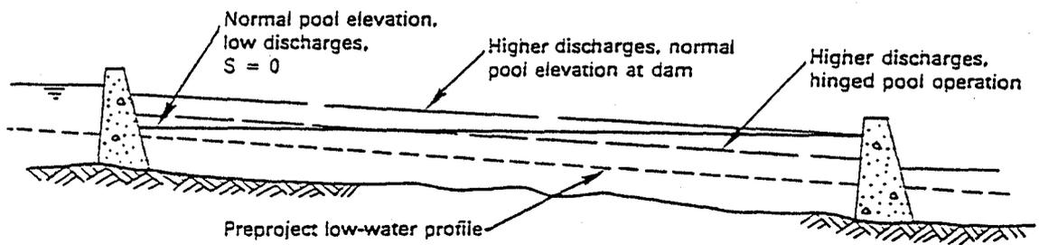
**Figure 6.1 Effect of pool operation on water surface elevations.**
