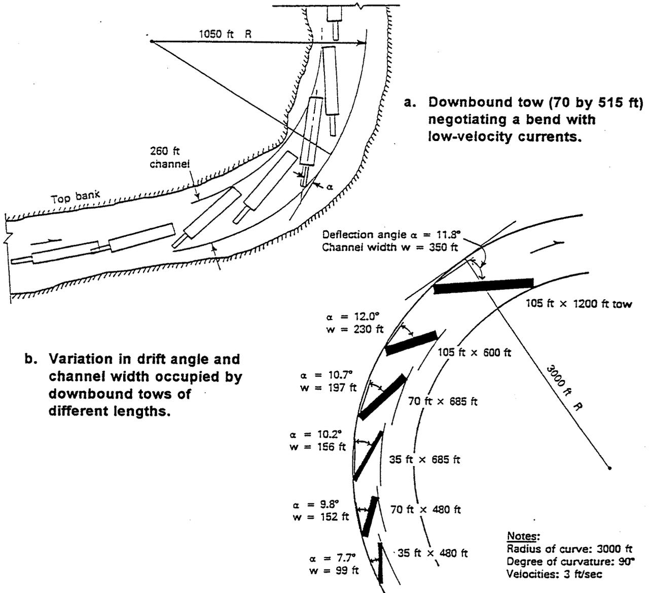
**Figure 5.2 Widths required in Bends.** (U.S. Army, Corps of Engineers, 1980)
