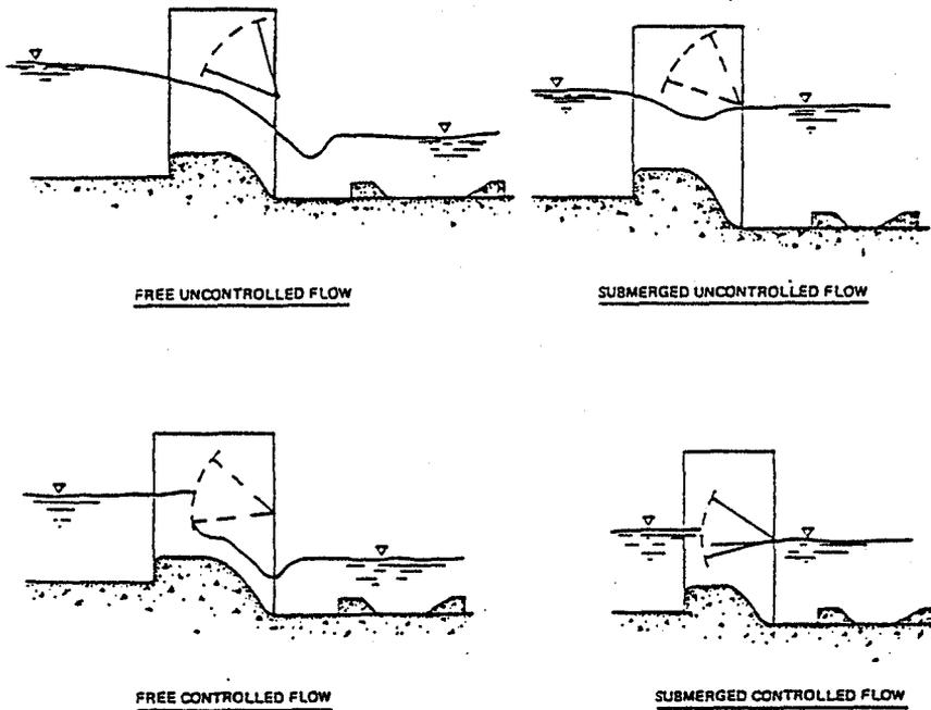
**Figure 7.5. Possible flow regimes, low-head navigation weirs.
