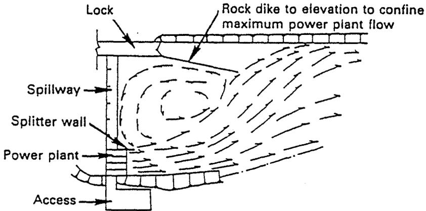
**Figure 9.24. Dike to minimize effect of power plant releases on navigation in lower lock approach, Dardanelle Lock and Dam, Arkansas River (Franco, 1976).**
