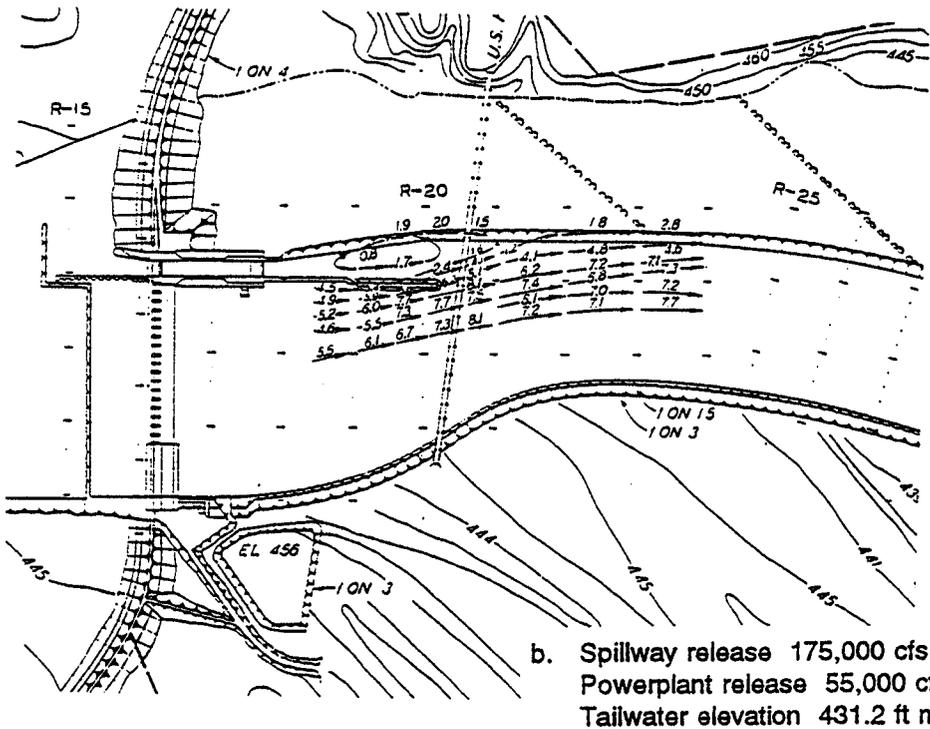
**Figure 9.7. Velocities and currents, lower lock approach, with modifications to improve navigation conditions, Robert S. Kerr Lock and Dam, Arkansas River (Franco and Glover, 1968).**
