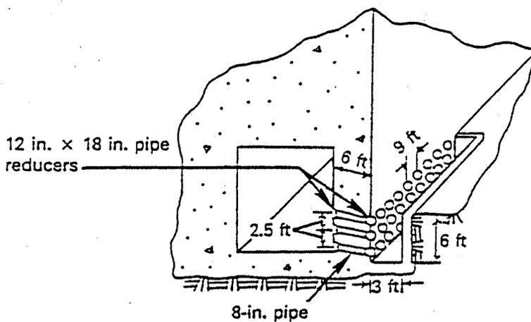
Figure 8.31. TVA multiport system (Elder et al., 1964).
