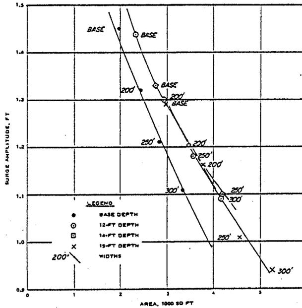
Figure 9.21 Maximum computed surge magnitudes at upstream end of transition above lock (Huval, 1980).
