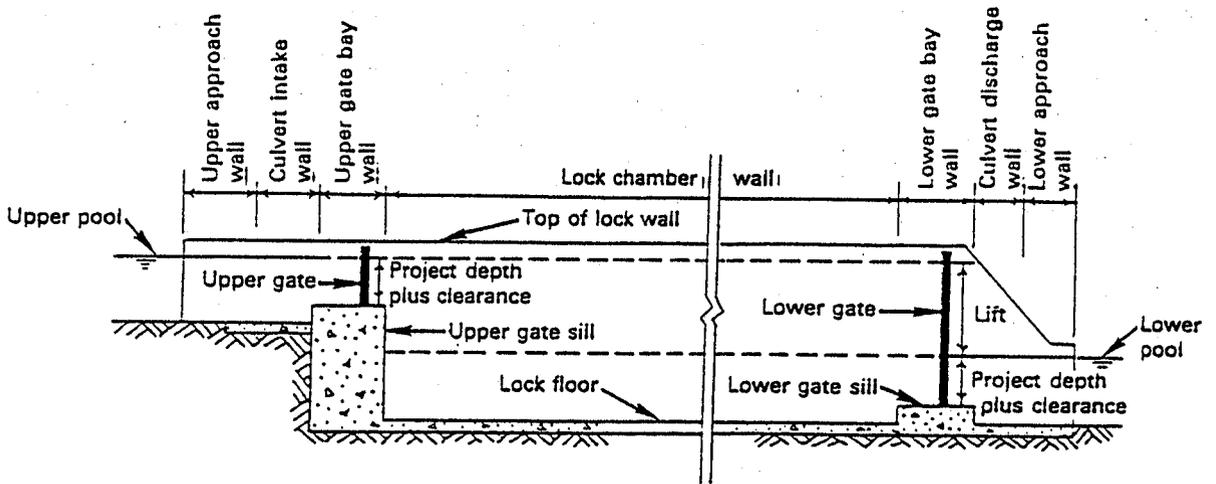
**Figure 8.9. Lock walls, gates, and sills.**
