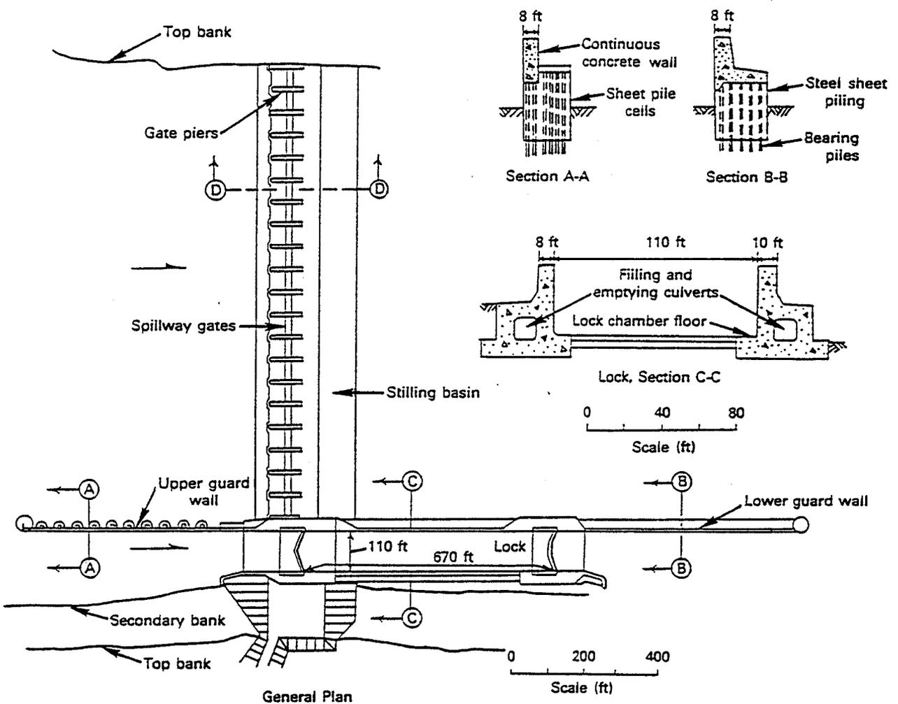
Figure 8.2 Typical low-lift navigation lock and dam (Ables and Boyd, 1966).
