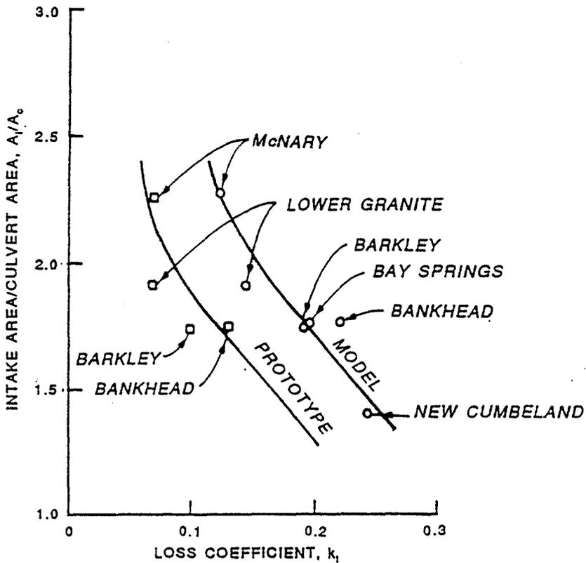
Figure 8.22. Intake head loss coefficient (Davis, 1989).
