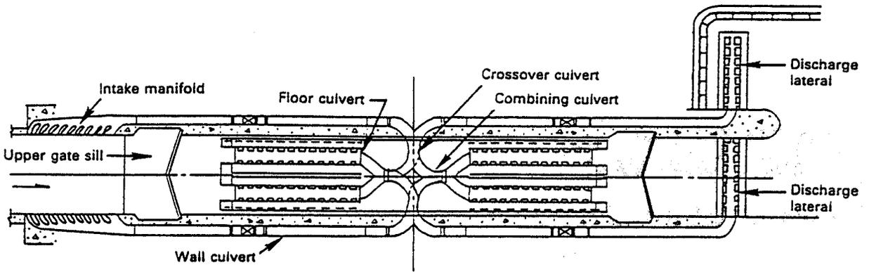
**Figure 8.39. Bottom longitudinal "over-and-under" filling and emptying system, Bay Springs Lock, 84-ft lift, Tennessee-Tombigbee Waterway. (Ables, 1978).**
