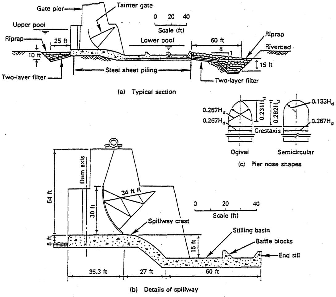
Figure 7.3 Typical non-navigable movable dam (gated spillway), Arkansas River. (Grace, 1965)
