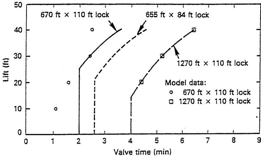
Figure 8.27. Recommended prototype valve opening times for filling (Murphy, 1975).
