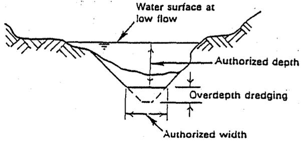
**Figure 10.1. Authorized channel dimensions and overdepth dredging for advance maintenance.**
