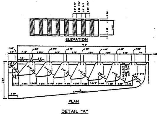
c. Alternative II, Intake canal and manifold.
