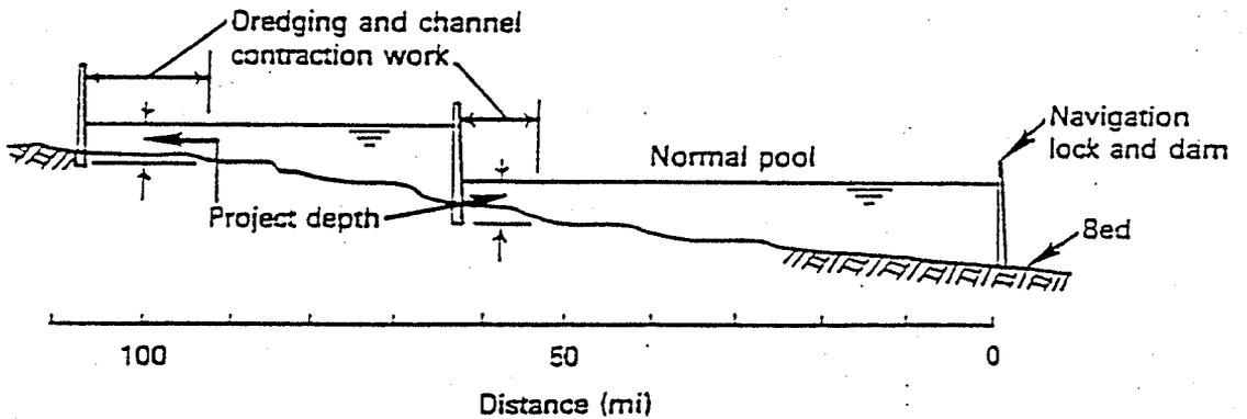
Figure 4.2 Typical location of dredging and contraction work at heads of pools.
