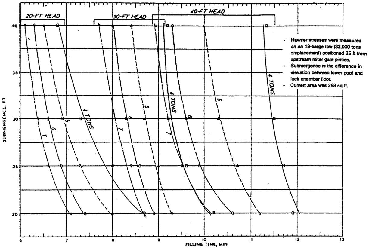
Figure 8.15. Permissible filling time to keep hawser stresses within 4-, 5-, 6-, and 7-ton limits, 110- by 1200-ft lock.
