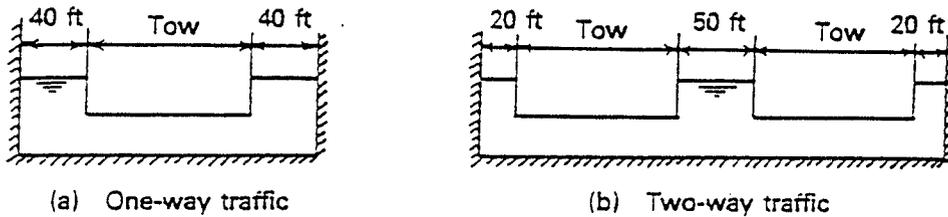
**Figure 5.1 Minimum channel clearance in straight reaches.**
