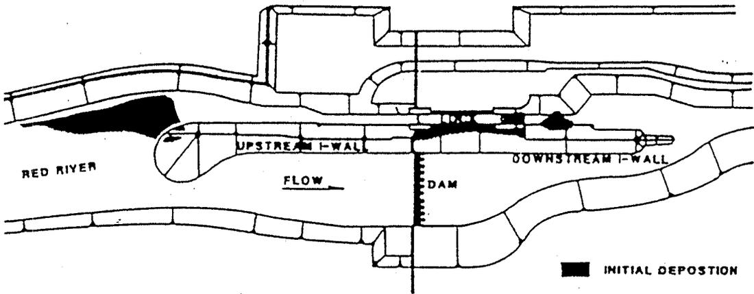
**Figure B.2, Initial deposition problem areas Lock and Dam 1, Red River Waterway. (Little, 1987).**
