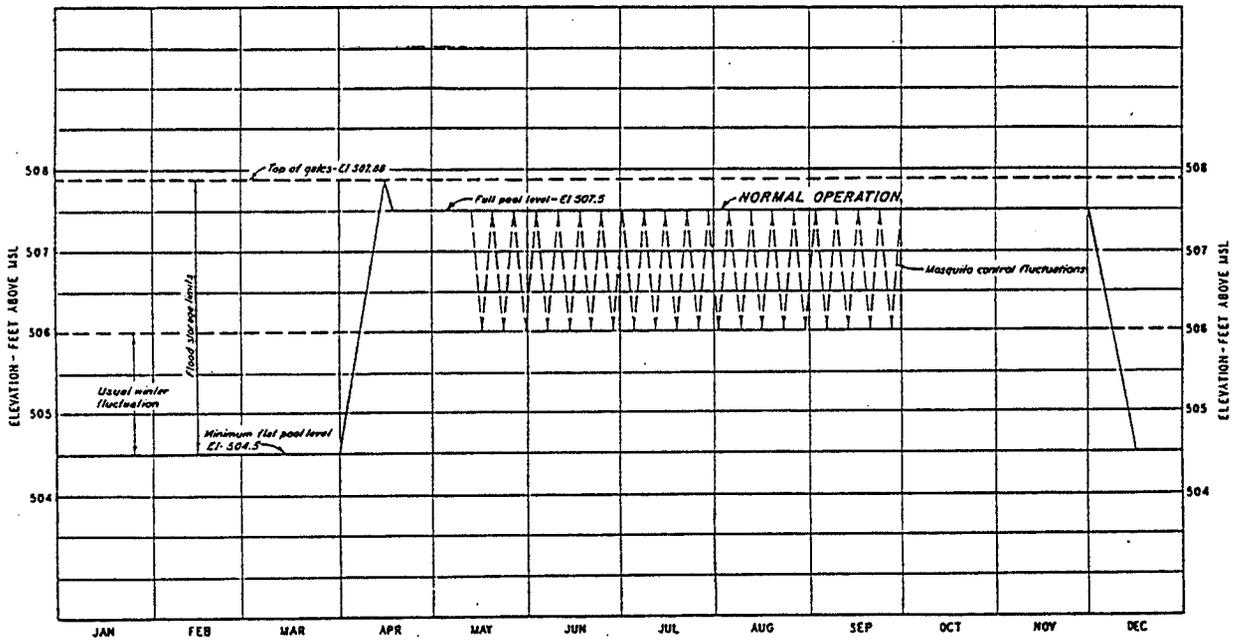
**Figure 6.2. Multiple-Purpose Reservoir Operation for Vector Control,
