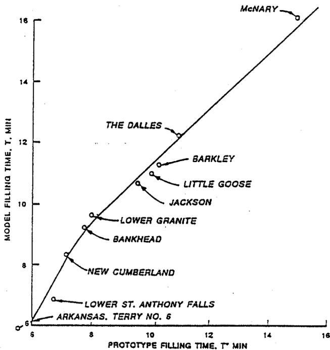
Figure 8.14. Prototype vs model filling time.
